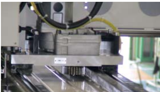
KRG Ground Rack and SSG Ground Spur Gear used as a work conveying device of the auto loader.
