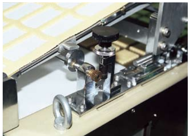
SW Worms and BG Worm Wheels used in adjusting a cloth feeding device
