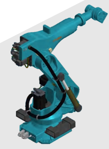
GD27180A Specified Load 180Kg Maximum Arm Span 2720mm
