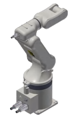
GD0805A Specified Load 5Kg Maximum Arm Span 800mm
