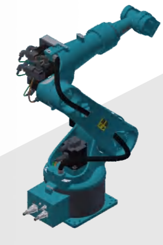
GD2380A Specified Load 80Kg Maximum Arm Span 2302mm
