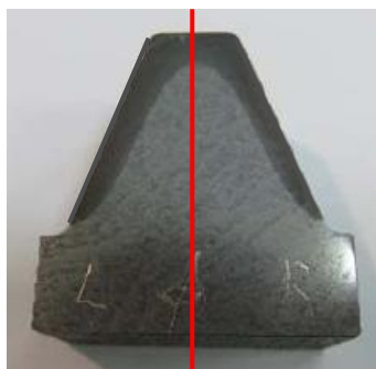
Qualified induction hardening and teeth grinding
